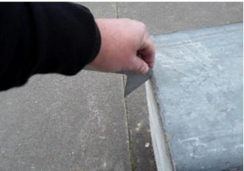
**Finding:** The item has exposed edges and corners with a radius of less than 3mm and fails the requirements of BS EN 14974
