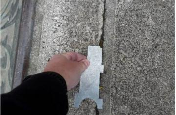
**Finding:** Joints between the riding surfaces should not be greater than 5mm to meet the requirements of BS EN 14974 between the joints do not exceed 5mm
